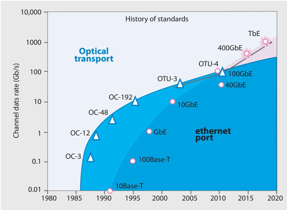
Figure 2: Data port speed and transport channel capacity evolution and predictions
