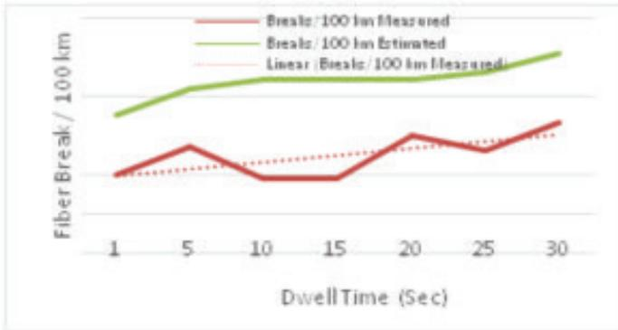
Figure 2 Estimated vs Measured fiber break rate
