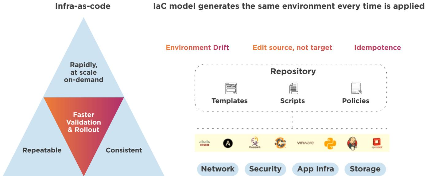
Infrastructure as Code (IaC) is the management of infrastructure (networks, virtual machines, load balancers and connection topology) in a descriptive model using DevOps methodology
