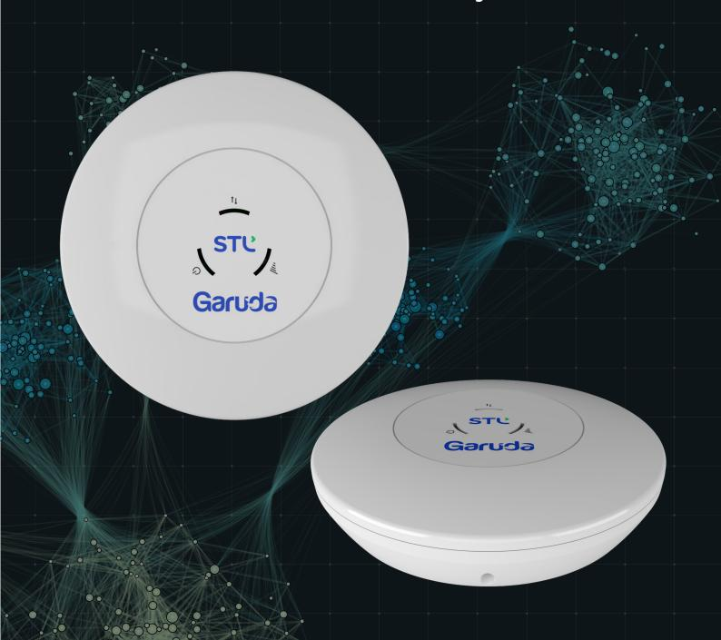
Garuda, an ORAN 7.2x split Indoor small cell which can truly enable 5G for every corner of residentials, enterprises etc. STL has indigenously designed and developed this radio to complement the network capacity, density and coverage of macro networks seamlessly.
