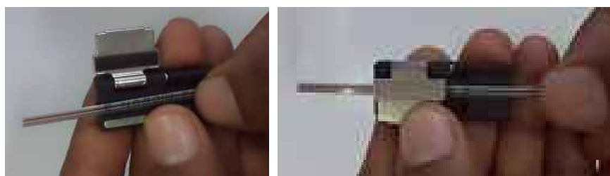
Figure 5- Placing of Fiber Ribbon in holders
