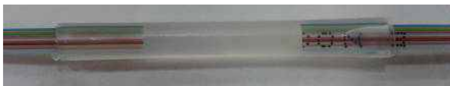
Figure 15- Spliced ribbon fiber with protection sleeve
