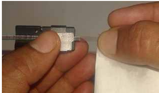
Figure 9a- Cleaning of stripped fiber
