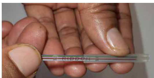
Figure 3- Splice protect heat shrink sleeve
