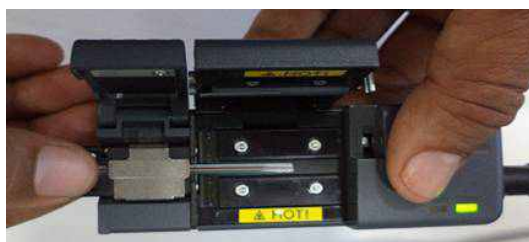
Figure 7- Placing the holder in Hot jacket stripper/thermal stripper
