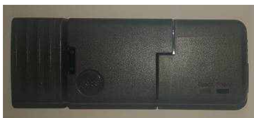
Figure 6- Hot jacket stripper/thermal stripper
