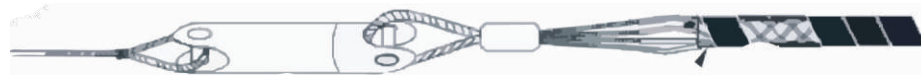
Figure 16 – Traveler supported at dead-end point to provide smooth feed of ADSS cable.
