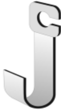
Figure 14 – "J" Hook used as a temporary support for ADSS Cable Moving Reel placing method. It is usually bolted to the support structure.
