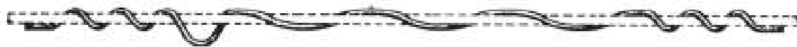
Figure 19 - Aeolian Vibration Damper used to induce a higher order of cable vibration.
