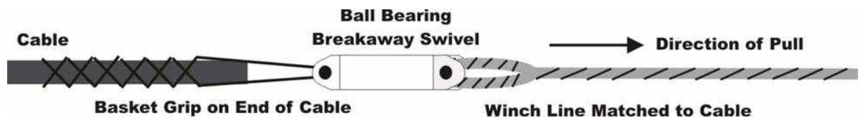
Figure 35- Cable Placement Array Using Ball-Bearing Swivel to Connect Winch Line to Cable
