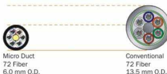
Figure 5– Comparison of Sterlite's Micro-Duct Optical Cable to a 72 Fiber Conventional Optical Cable
