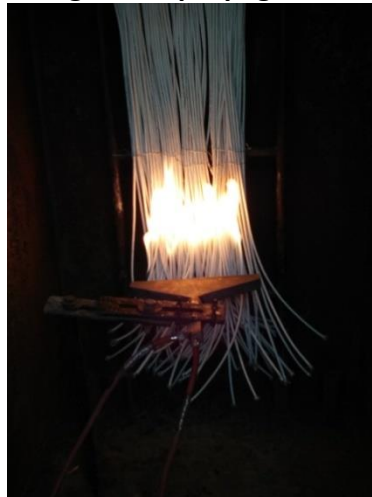
During Flame propagation test
