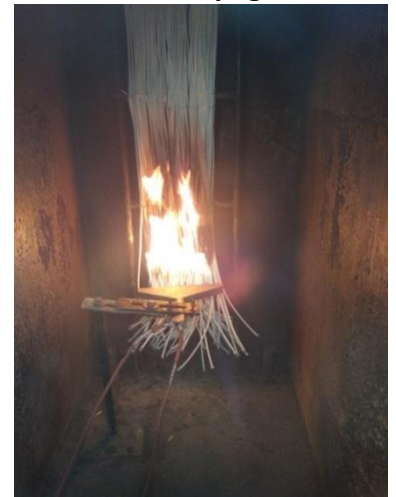
After Flame Propagation test
