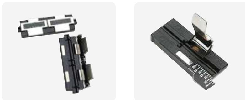
*Figure 5- Ribbon Holding Block, Used to Position Ribbons during Cleaving and Splicing. Different Blocks are Available for 12 and 24 Fiber Ribbons.*
