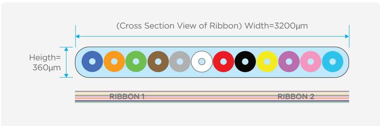
Figure 1- Cross-Sectional View and Plan View of Sterlite 12 Fiber Ribbon
