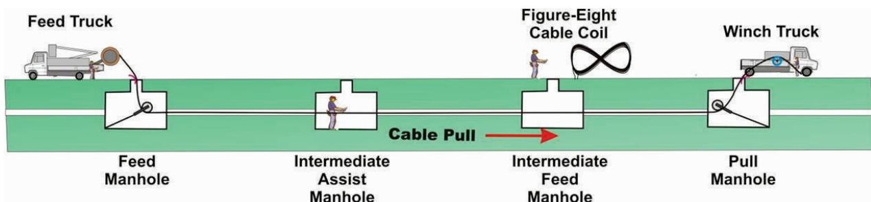
Figure 1 – Schematic Showing Different Types of Manholes
