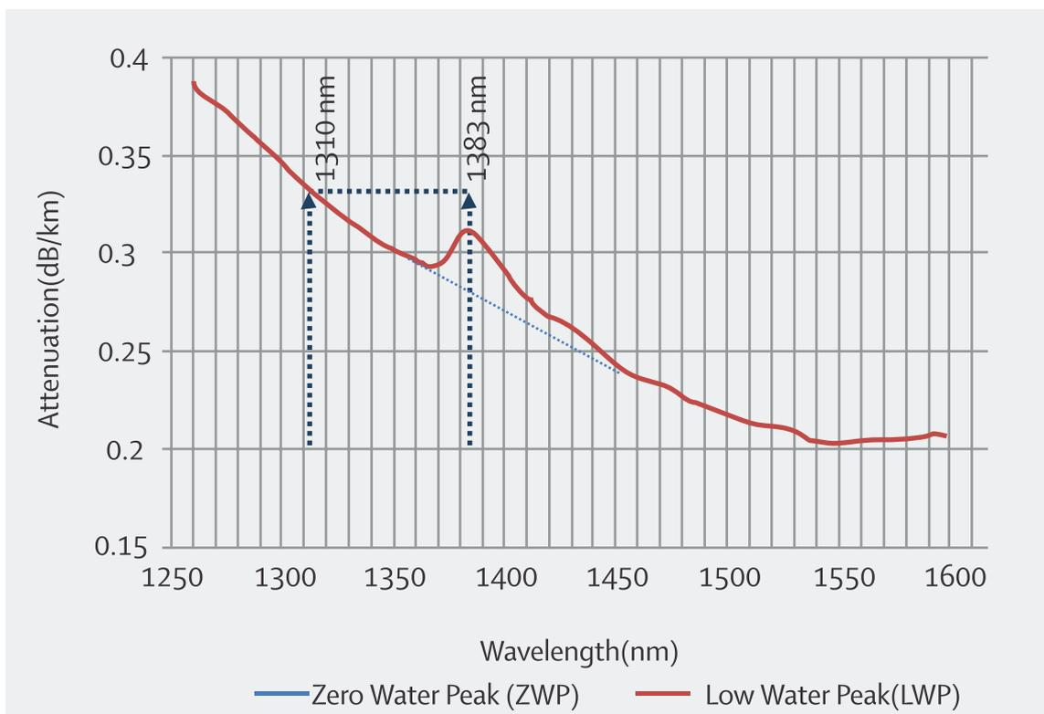
**Figure 1 Typical Spectral attenuation plot of Zero and Low Water Peak fiber**
